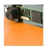
A carrier card integrates a processor system (SOM-module) with a separate Image sensor board. The modular approach makes it simple to adapt for new sensors.
